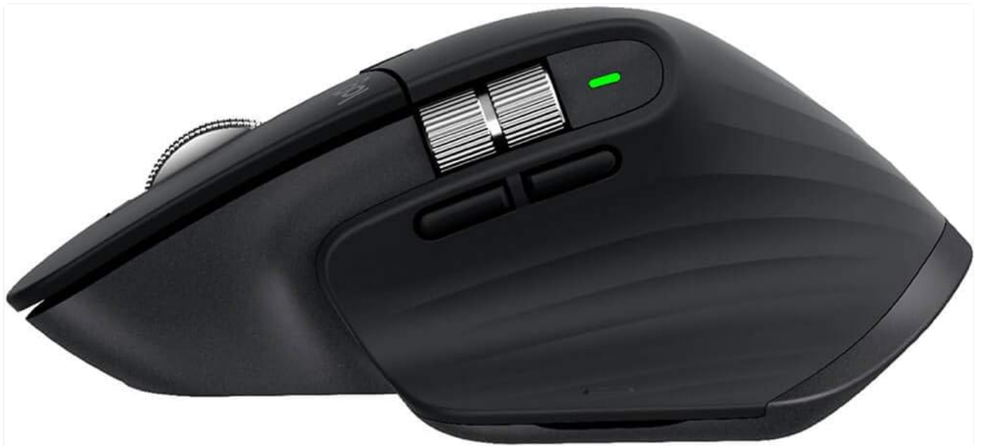
Figure 4: Main Scroll Wheel and Mode-Shift Button. This image shows the primary scroll wheel and the button used to switch between ratcheted and hyper-fast scrolling modes.
