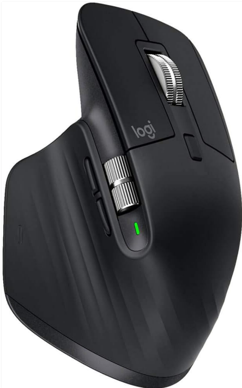
Figure 5: Thumb Wheel and Side Buttons. This image illustrates the thumb wheel for horizontal scrolling and the customizable forward/back buttons.
