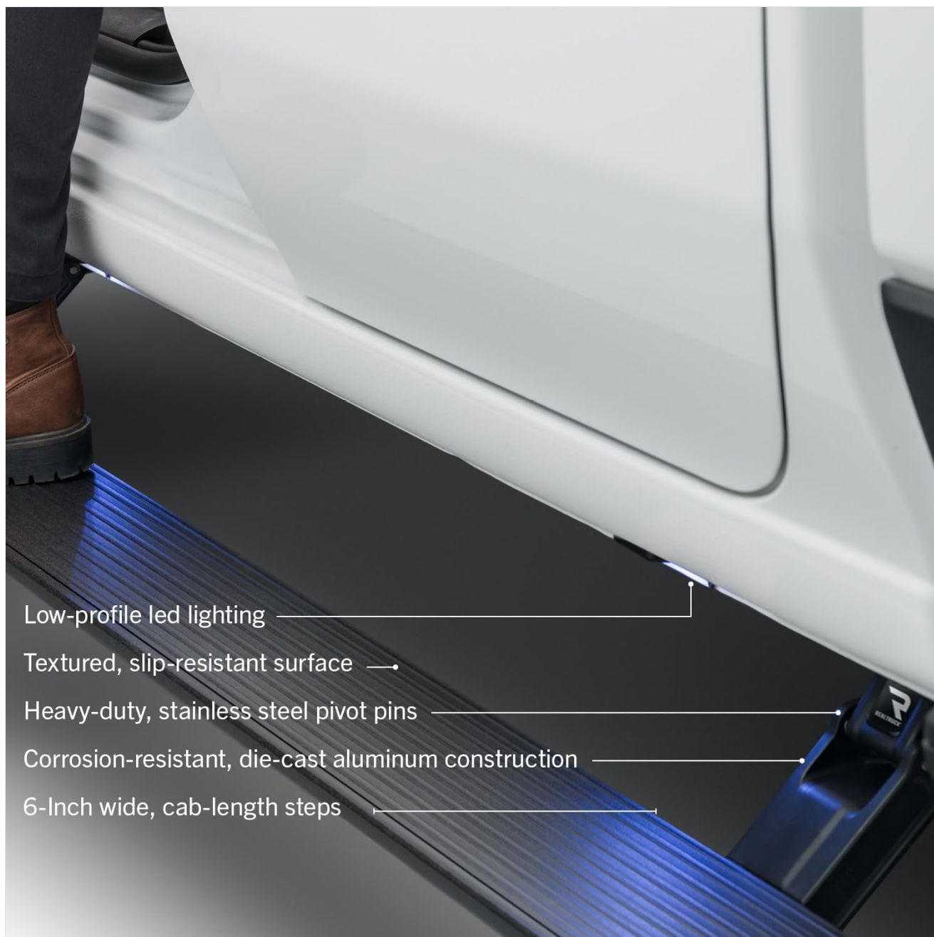
Image 5.2: The PowerStep featuring low-profile LED lighting for improved visibility and a textured, slip-resistant surface.
