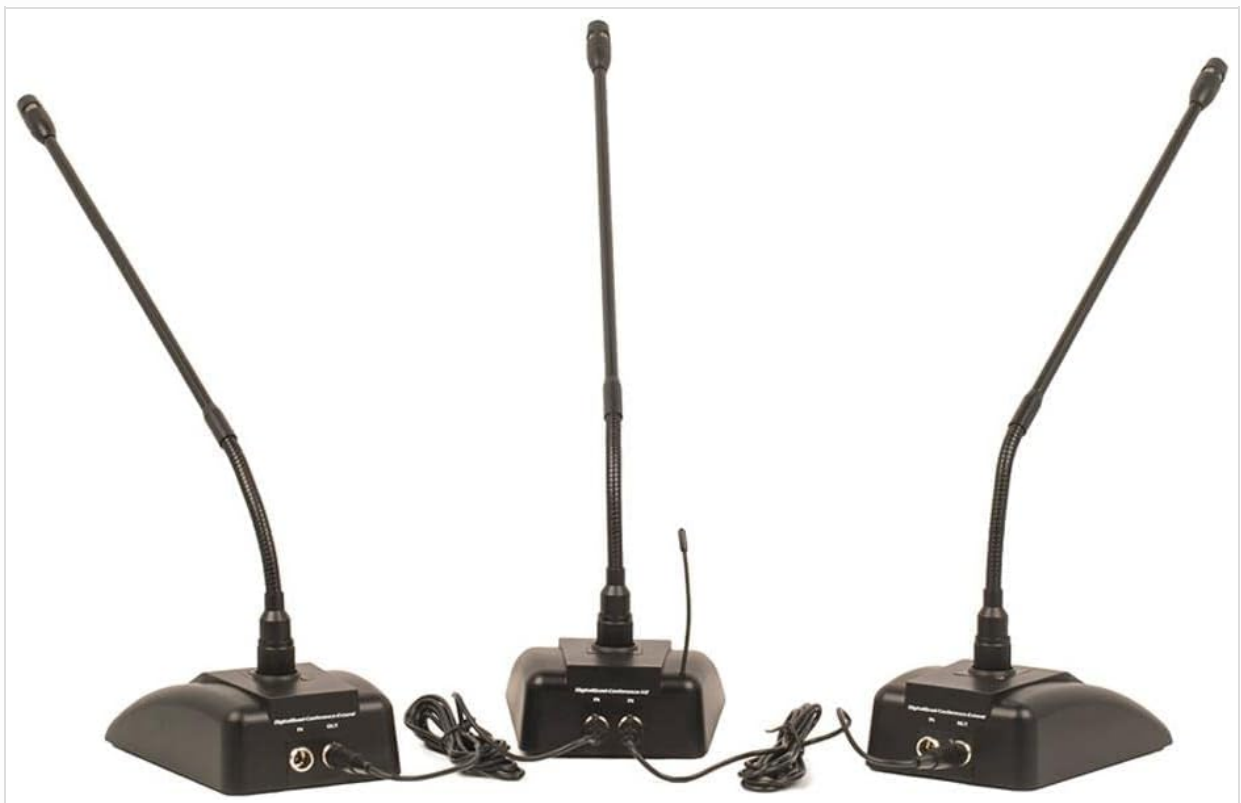
Image: Three microphone bases demonstrating wired expansion. The "OUT" port of one base is connected to the "IN" port of the next, allowing multiple wired microphones to share a single wireless channel.
