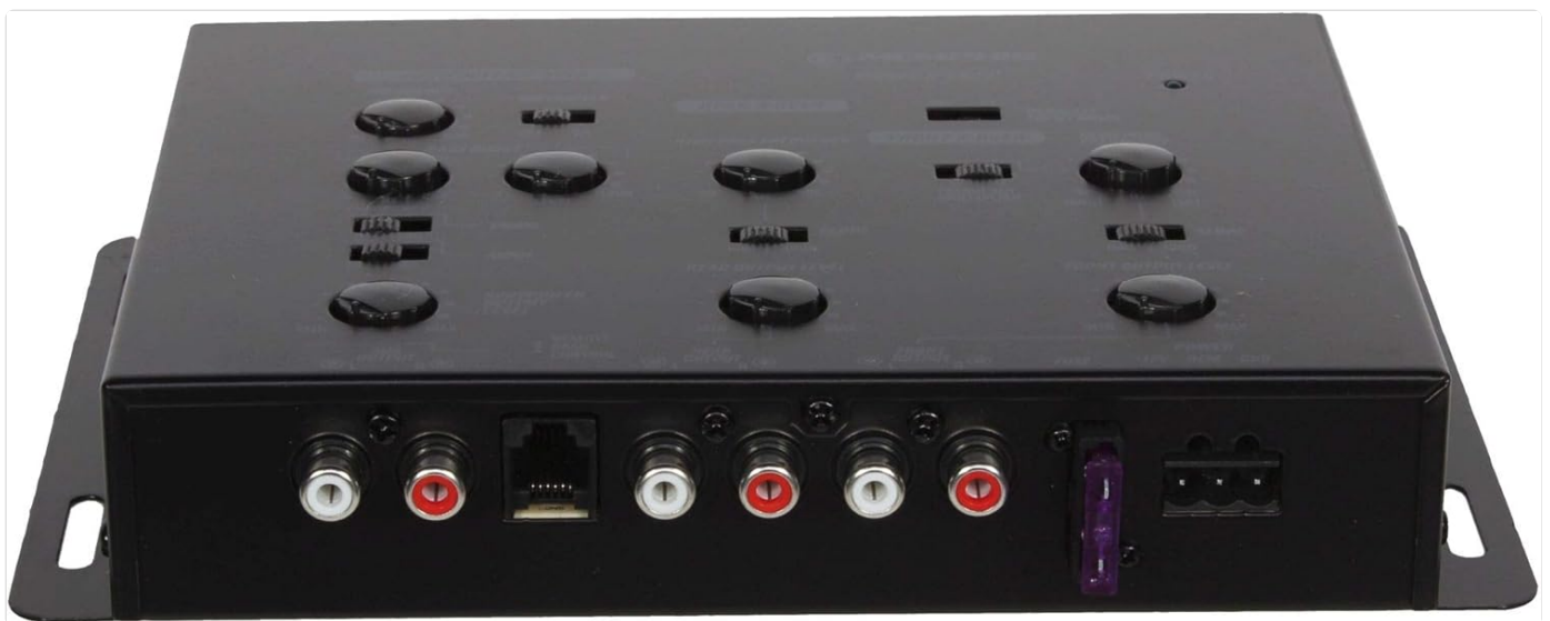
Figure 2: Rear panel of the Memphis Audio CX23 showing input and output RCA connections, remote bass control port, and power terminals.
