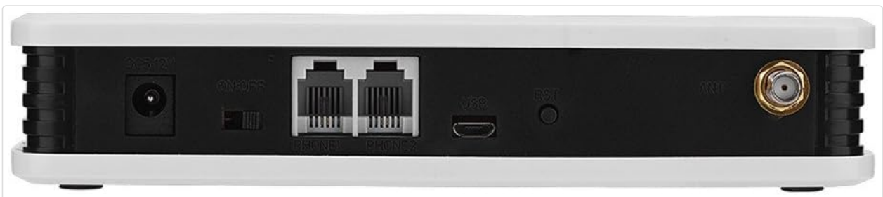
Figure 1: The GSM Fixed Wireless Terminal can connect to various communication products like telephones, alarm boxes, and recorders.
