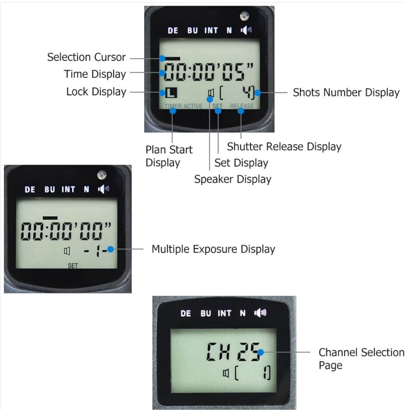
Image 2.3: The LCD display showing Selection Cursor, Time Display, Lock Display, Shots Number Display, Plan Start Display, Shutter Release Display, Set Display, Speaker Display, Multiple Exposure Display, and Channel Selection Page.
