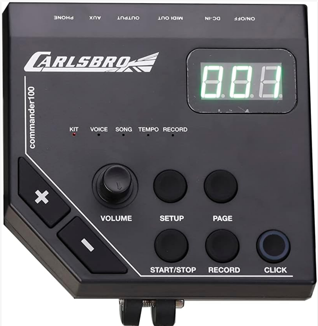
Image: Close-up view of the Commander 100 Sound Module, showing its display, buttons, and control knob.
