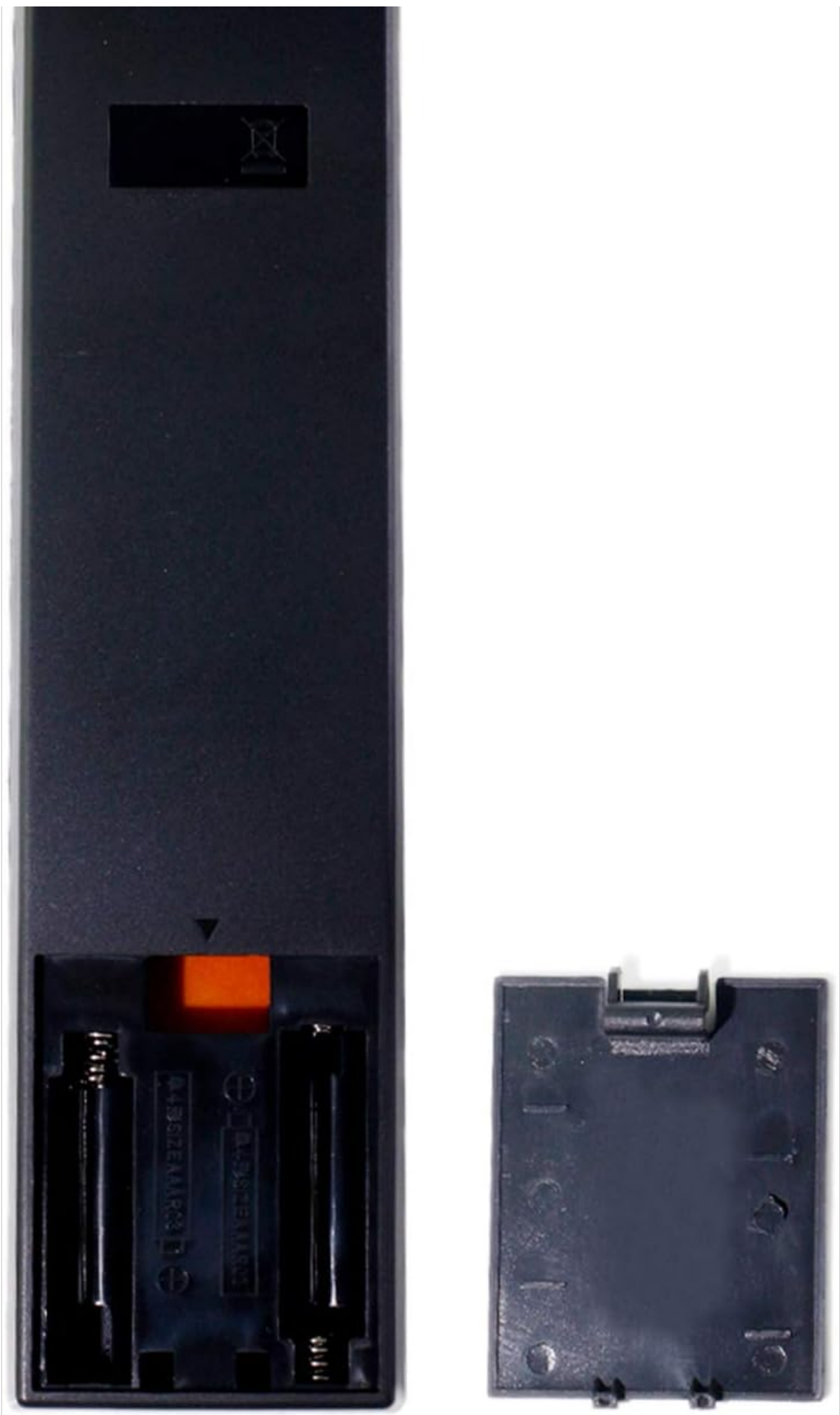
Image: Back of the remote control with the battery cover removed, showing the battery insertion slots.
