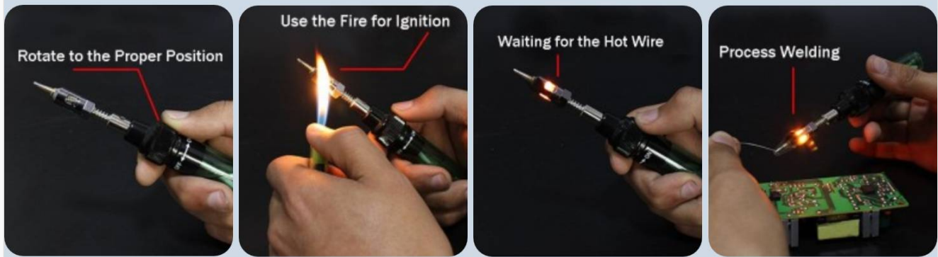
Figure 3: Ignition and soldering process.
