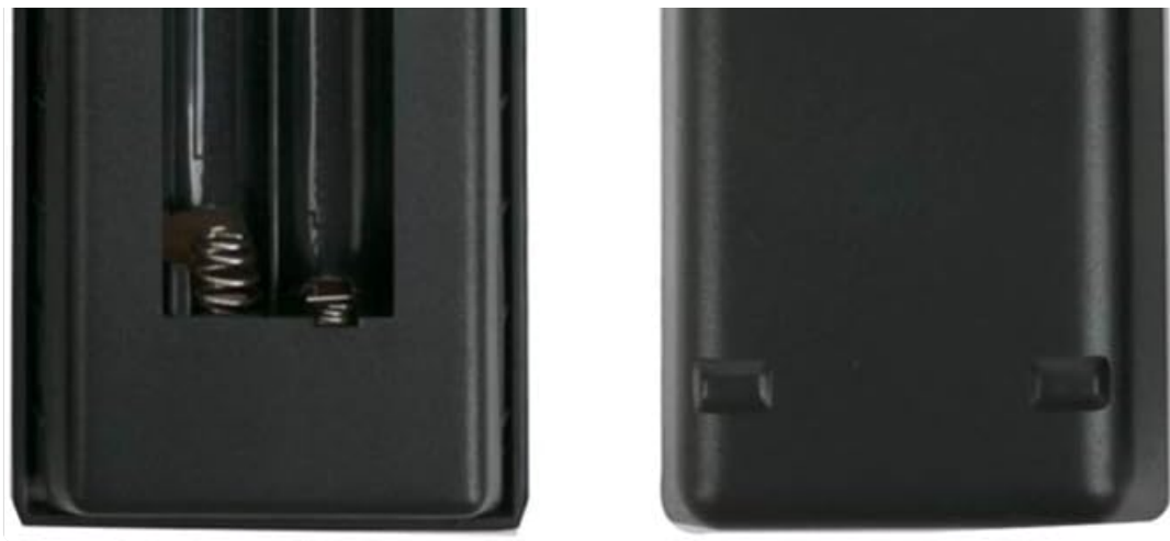
Image: Rear view of the remote control with the battery cover removed, revealing the battery slots. This illustrates where to insert the two AAA batteries.
