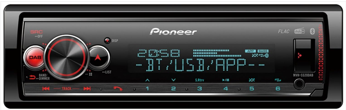
Figure 1: Front panel of the Pioneer MVH-S520DAB Digital Media Receiver. This image displays the main control knob, the DAB button, source selection (SRC) button, and the multi-color display.
