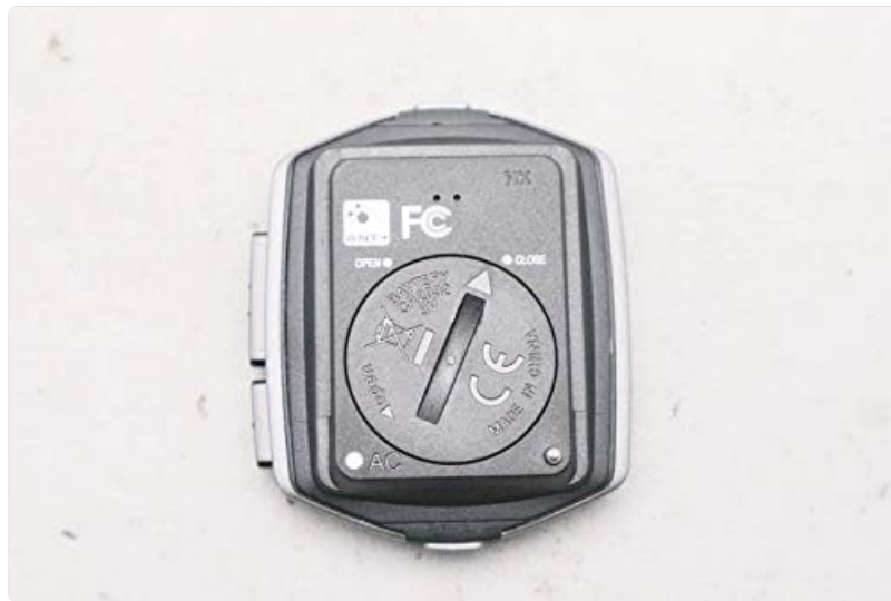
Figure 3.1: Rear view of the NODE2.1 unit, highlighting the battery compartment with "OPEN" and "CLOSE" indicators for battery installation or replacement.
