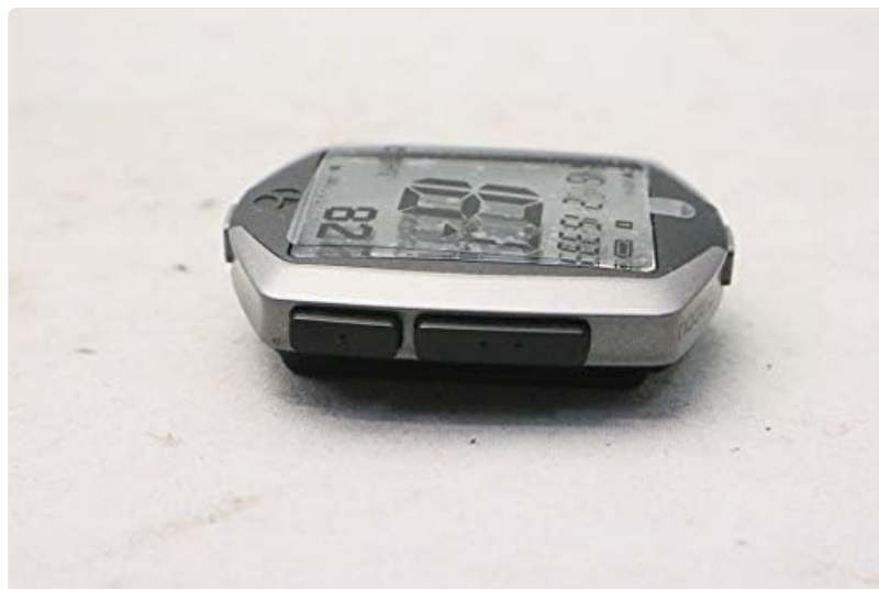
Figure 4.2: An alternative side view of the NODE2.1, highlighting the array of control buttons on the unit's side, used for navigation and function selection.
