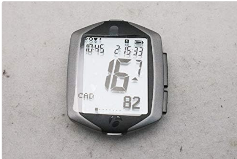
Figure 1.1: Front view of the BONTRAGER NODE2.1 Cycle Computer, showing the digital display with time, speed, and other metrics.
