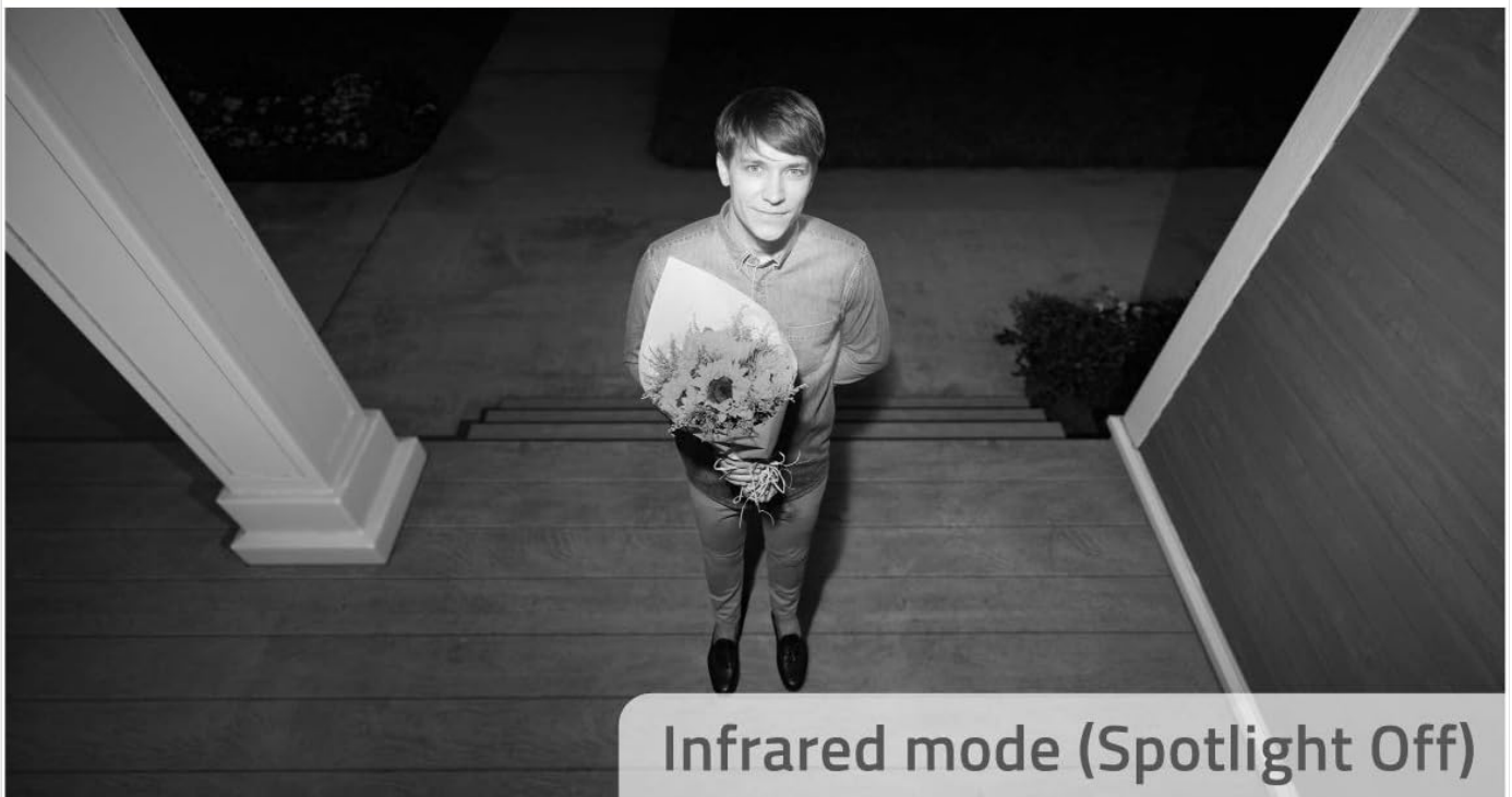
Figure 3.2: Night vision options include color mode with the spotlight activated and infrared mode for discreet monitoring.
