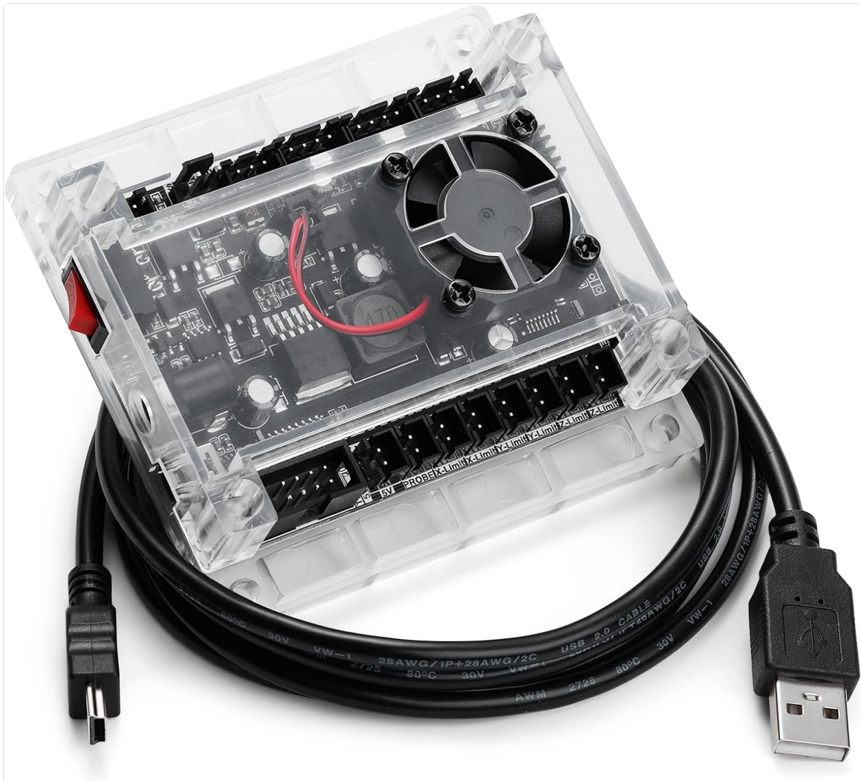
Image 2.1: The SainSmart Genmitsu CNC Controller Board, shown with its protective ABS case and an included USB cable for connection to a computer.
