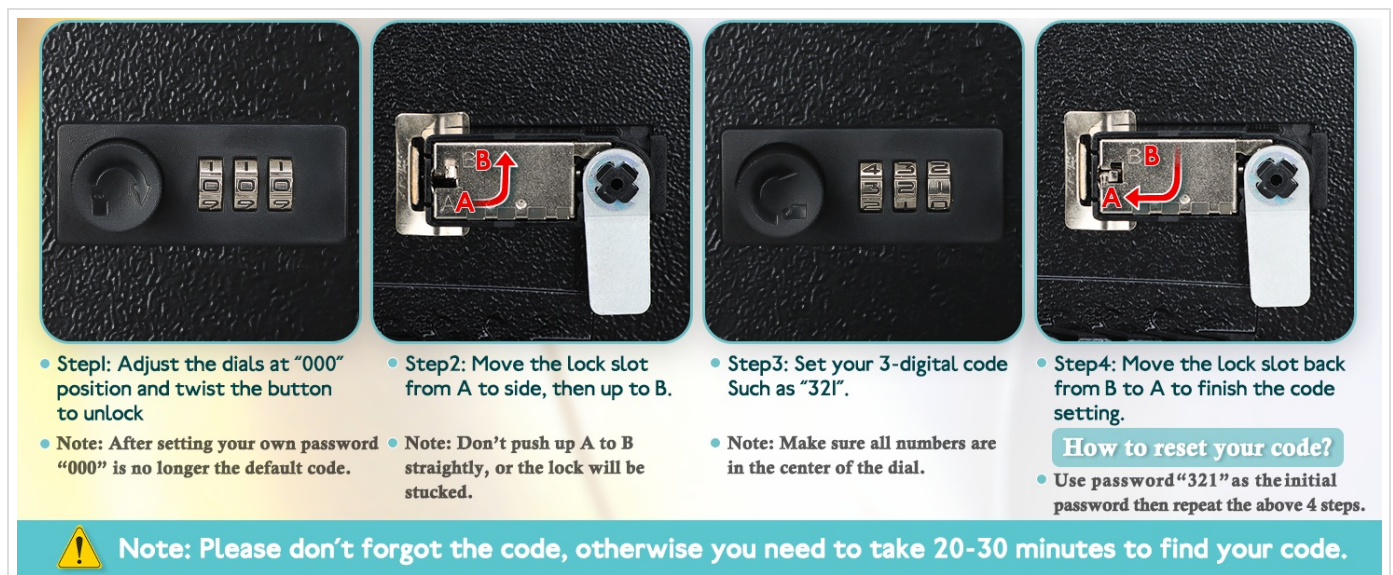
Image: Step-by-step instructions for setting and resetting the 3-digit combination lock.
