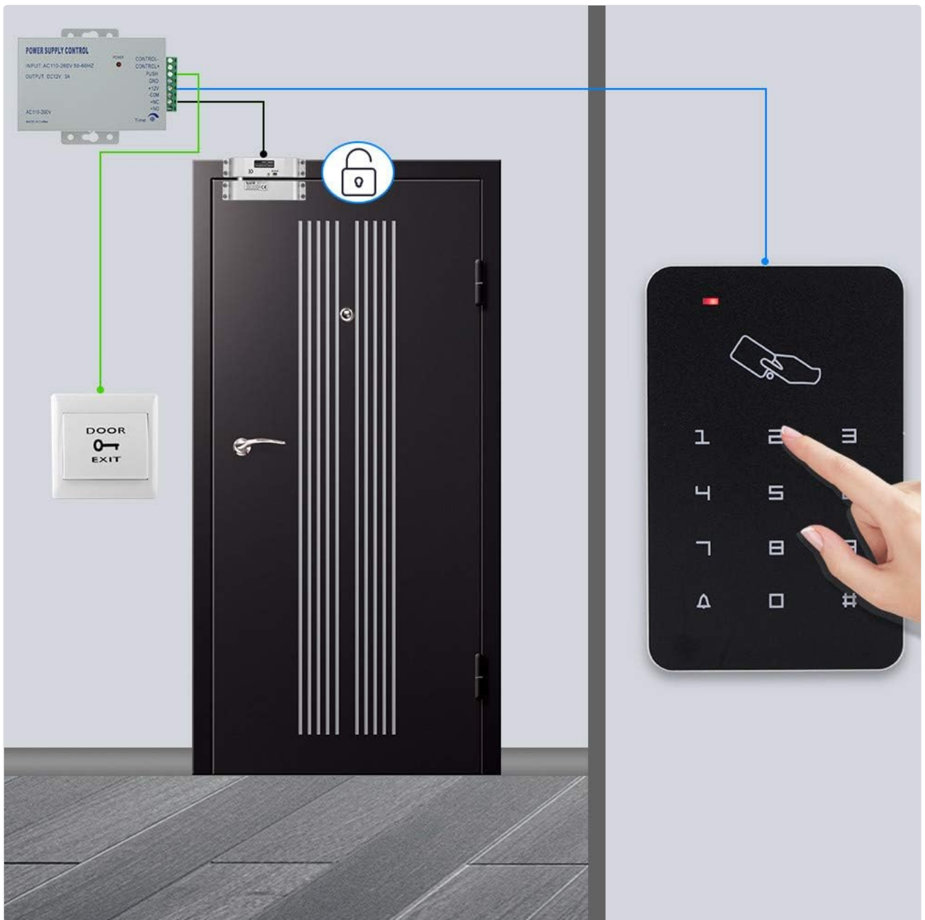
Figure 2.5: Complete Access Control System Diagram. A visual representation of the entire system connected to a door, showing the keypad, power supply, electric lock, and exit button in an operational setup.
