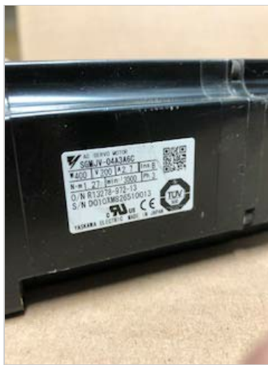
Figure 3.2: Side view of the Yaskawa SGMJV-04A3A6C AC Servo Motor, highlighting the product label. The label provides critical information such as the model number (SGMJV-04A3A6C), power (400W), voltage (200V), and other technical specifications.
