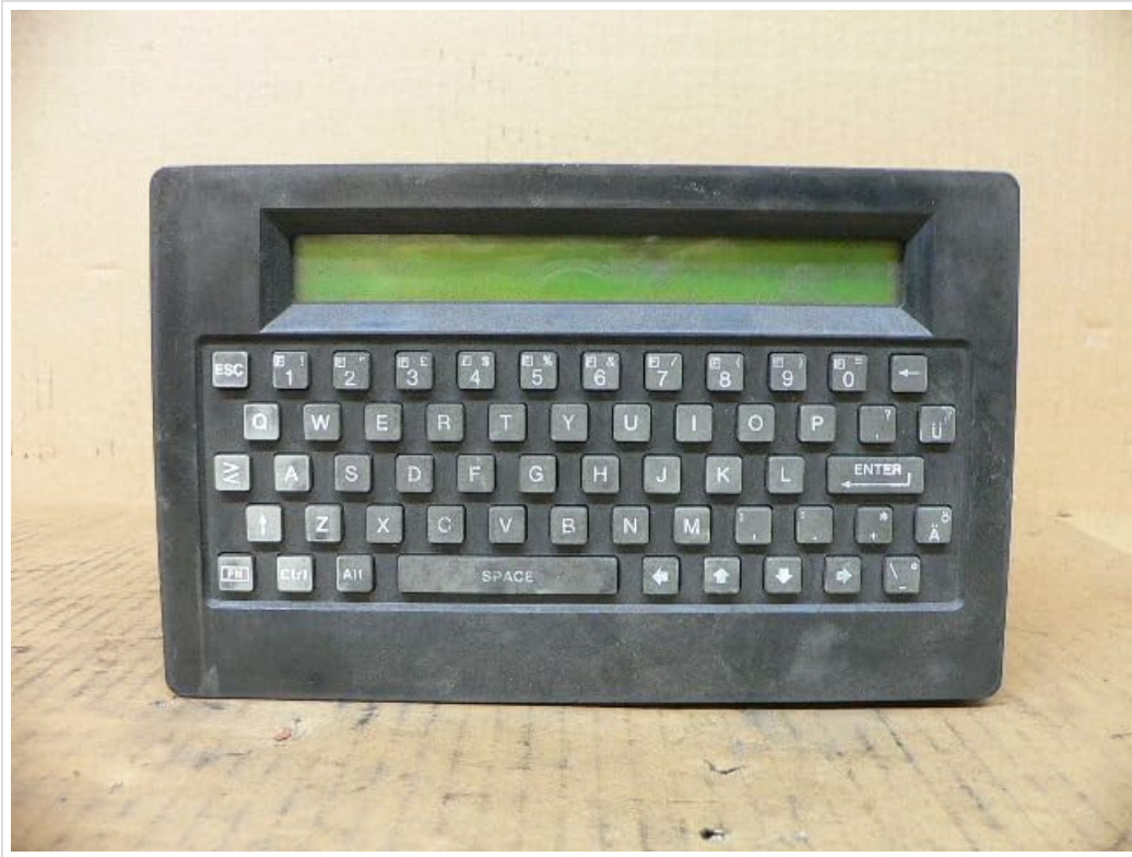
Figure 3.1: Front Panel. This image displays the front of the Sitel MK3-M8-3-BOX controller, featuring a green monochrome display screen at the top and a full QWERTY keyboard below it. The keyboard includes alphanumeric keys, function keys (ESC, ALT, CTRL), arrow keys, and an ENTER key. The casing is dark gray and appears to be made for industrial use.
