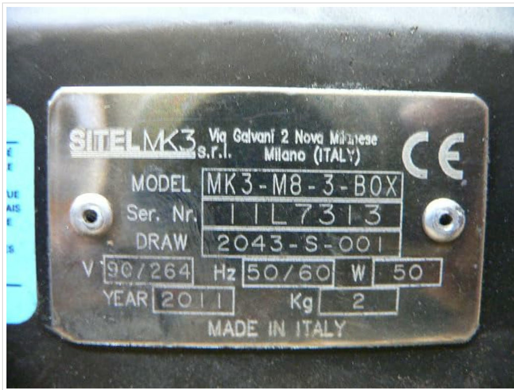
Figure 3.3: Product Nameplate. This close-up image displays the metallic nameplate affixed to the Sitel MK3-M8-3-BOX controller. It clearly shows the brand "SITELMK3", model "MK3-M8-3-BOX", serial number "11L7313", and electrical specifications including voltage (90/264 V), frequency (50/60 Hz), and power (50 W). The plate also indicates "MADE IN ITALY" and the manufacturing year "2011".
