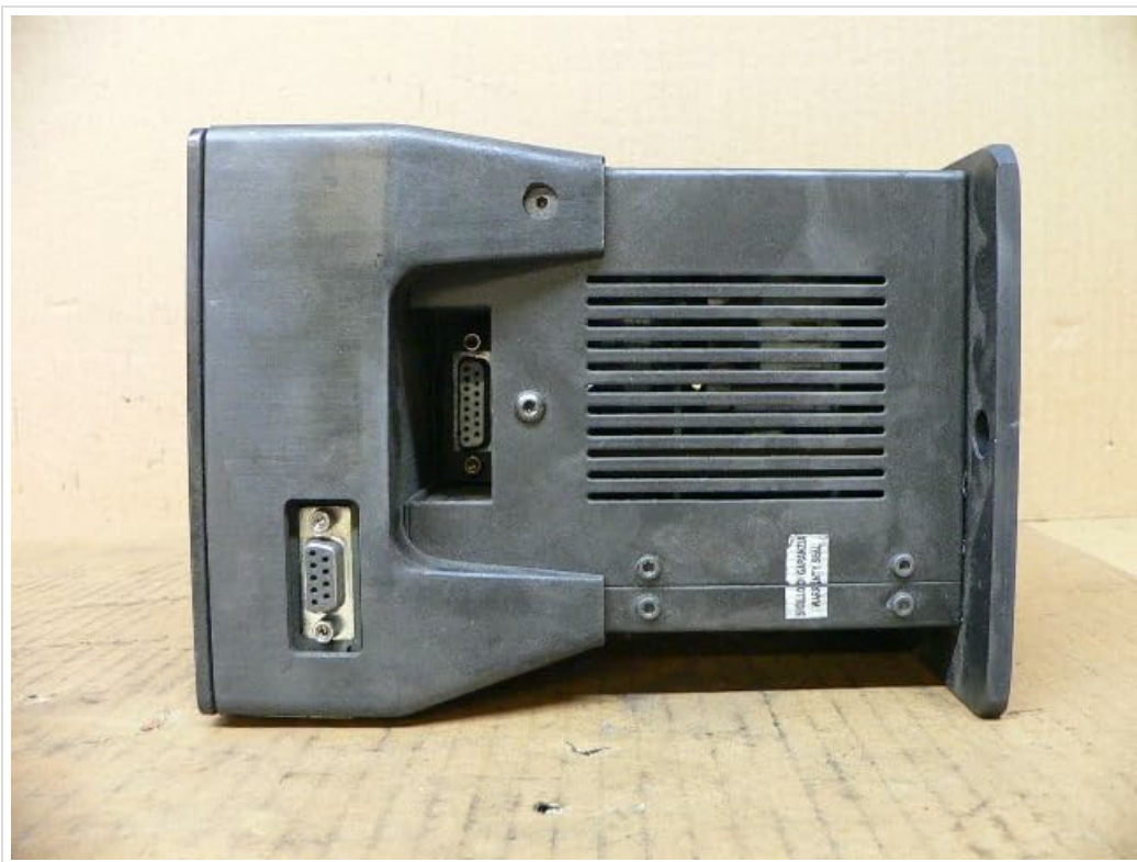
Figure 3.2: Side Panel. This image shows the side of the Sitel MK3-M8-3-BOX controller. Visible features include two D-subminiature connectors (likely serial ports) for external connections, and a series of ventilation grilles to dissipate heat. A small white sticker with text is also visible near the grilles, possibly indicating a warranty or inspection status.
