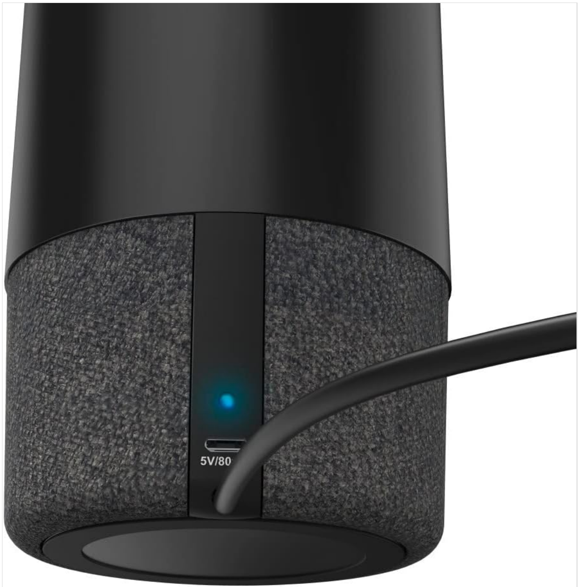
Image: A detailed view of the antenna's base, highlighting the USB power input and the blue LED indicator, which confirms the antenna is receiving power.
