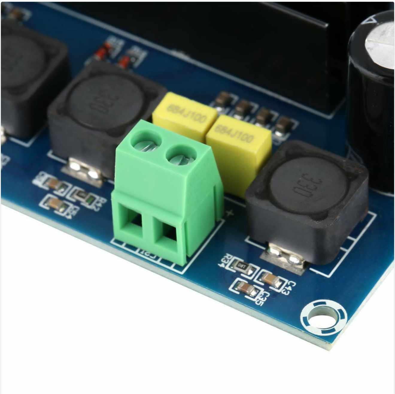
Figure 4.3: Detail of the speaker output terminals for connecting left and right channel speakers.
