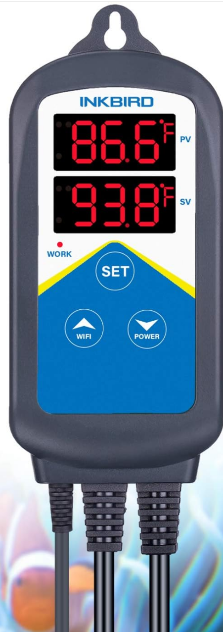
Figure 5: Close-up of the Inkbird ITC-306A display and control buttons, showing the current temperature (PV) and set temperature (SV).
