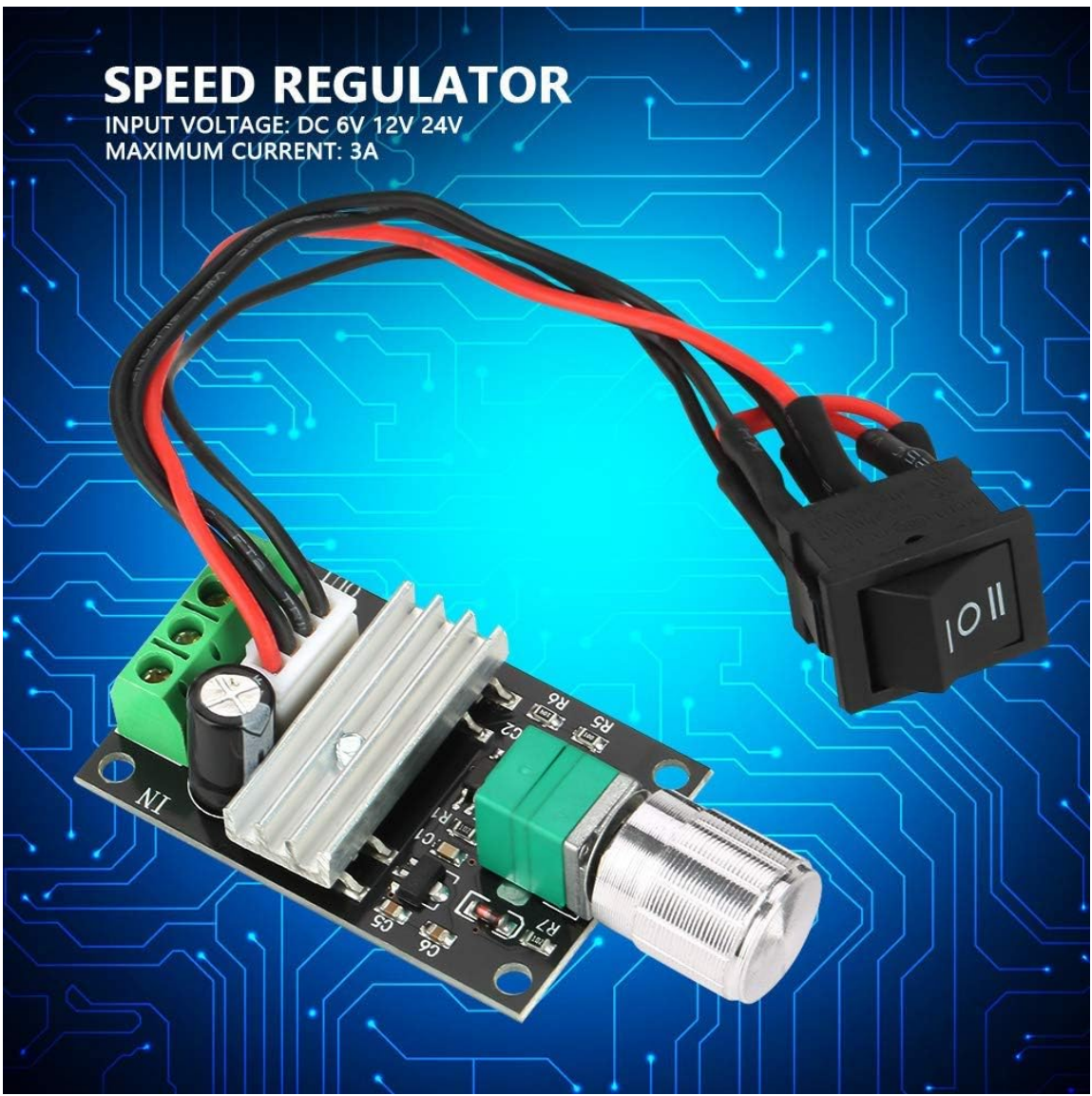
Figure 1: Overview of the DC Motor Speed Controller with connected wires and reversing switch. Note the 'IN' and 'OUT' terminals.
