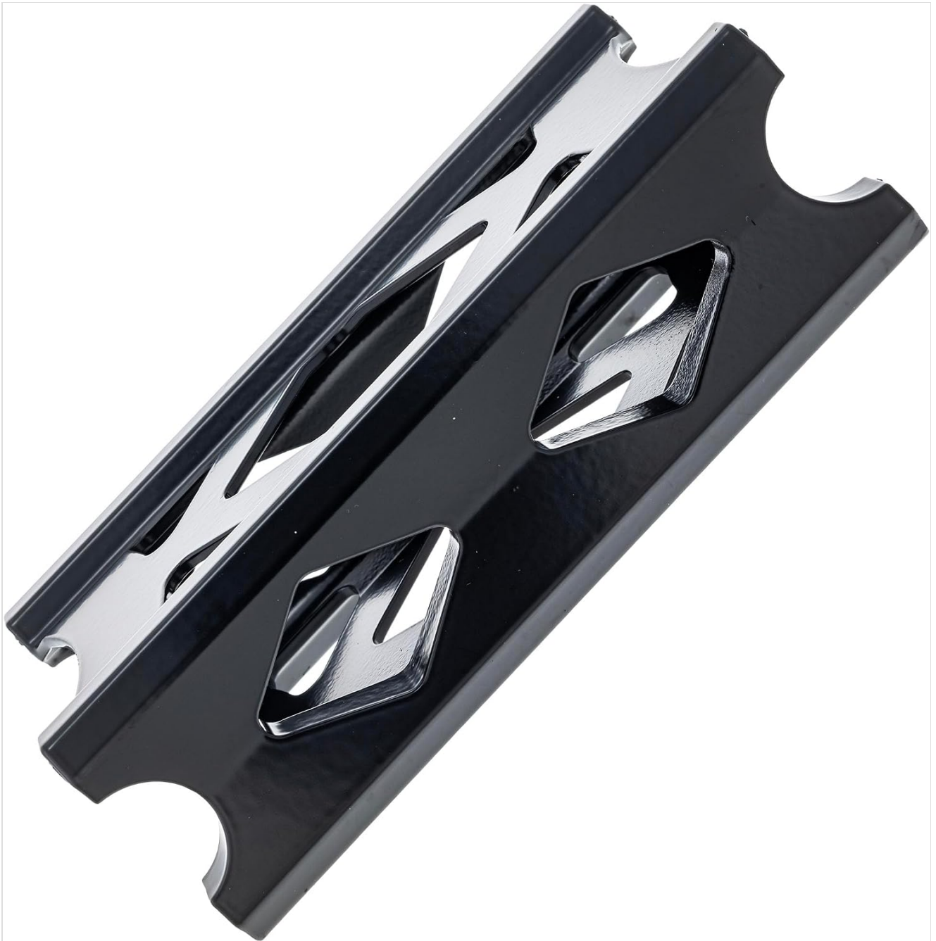
Image 5: Bottom view of the riser, showing the mounting points that connect to the snowmobile's steering post.
