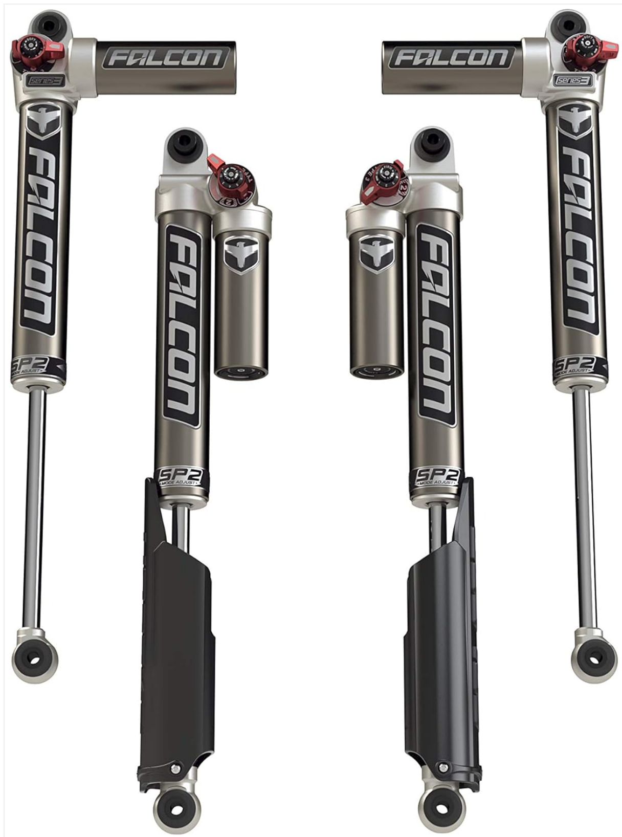
Figure 1: Falcon SP2 3.3 Fast Adjust Piggyback Shocks. This image displays four shock absorbers, each featuring a main body, a piggyback reservoir, and red adjustment knobs. The shocks are designed for vehicle suspension systems.
