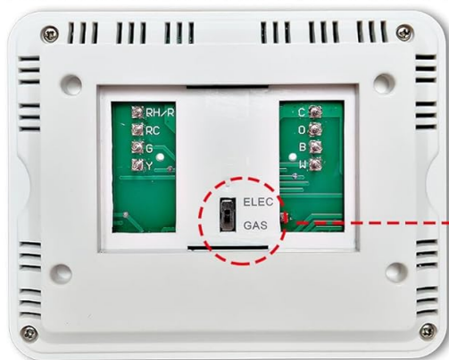
Image 5.1: Wiring diagram and system switch setting for the Suuwer S701 thermostat.
