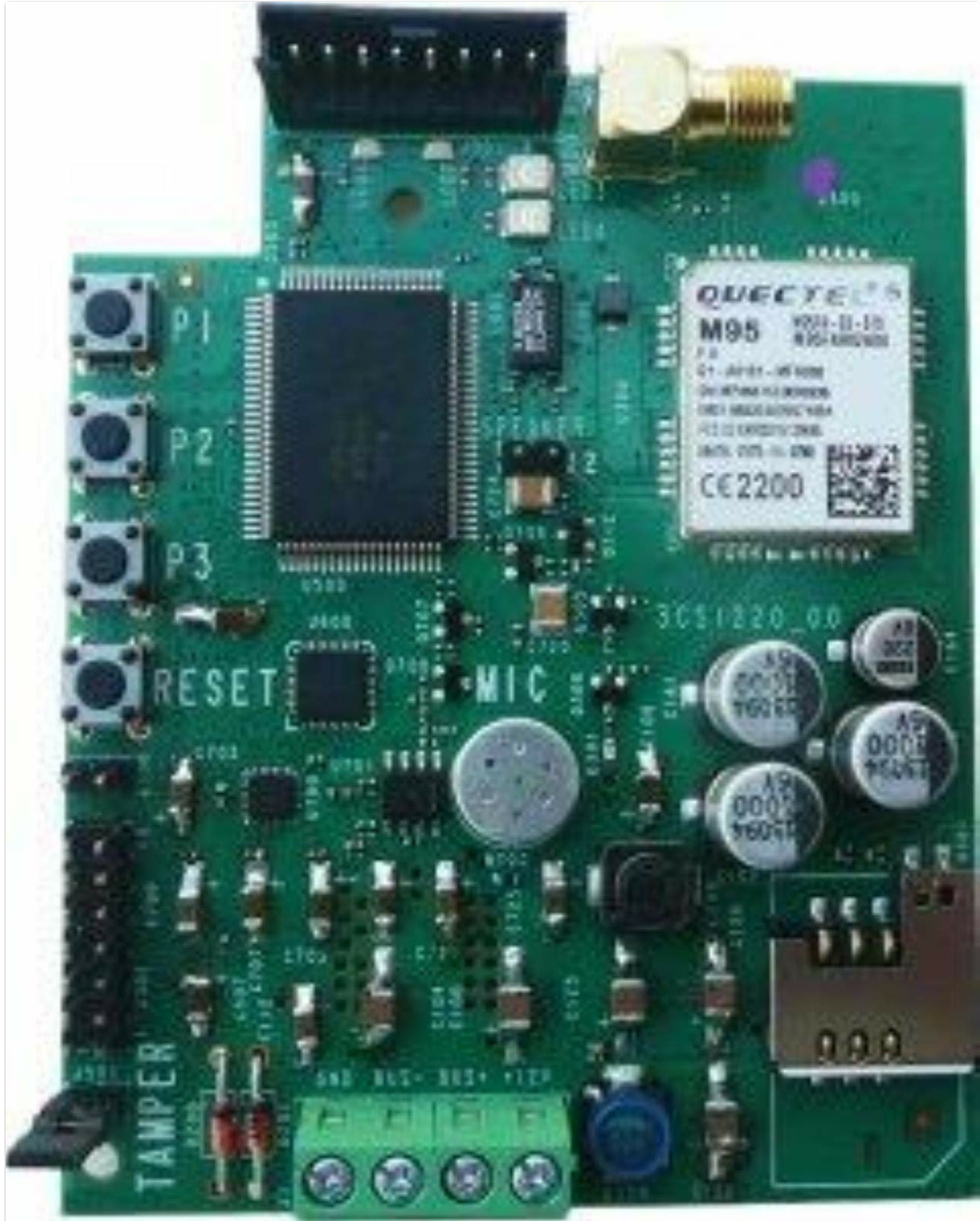
Figure 1: Front view of the Fracarro CT-Bus GSM Mini Telephone Combiner. The image displays the compact unit, typically showing the SIM card slot, antenna connector, and bus connection terminals.
