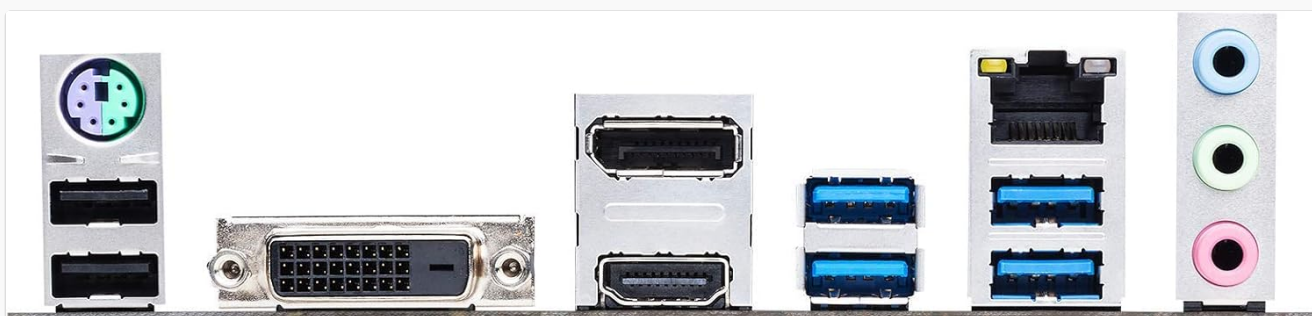
Close-up of the rear input/output (I/O) panel, displaying ports for USB, HDMI, DVI, LAN, and audio.
