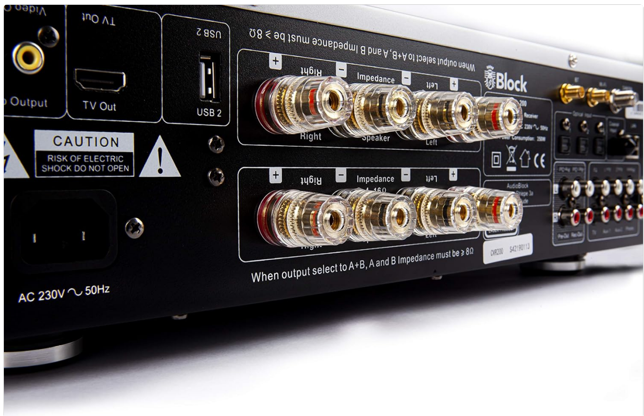
Image 4: Close-up of the speaker terminals. This detailed view focuses on the two sets of gold-plated speaker terminals (Speaker A and Speaker B) on the rear panel, designed for secure wire connections.
