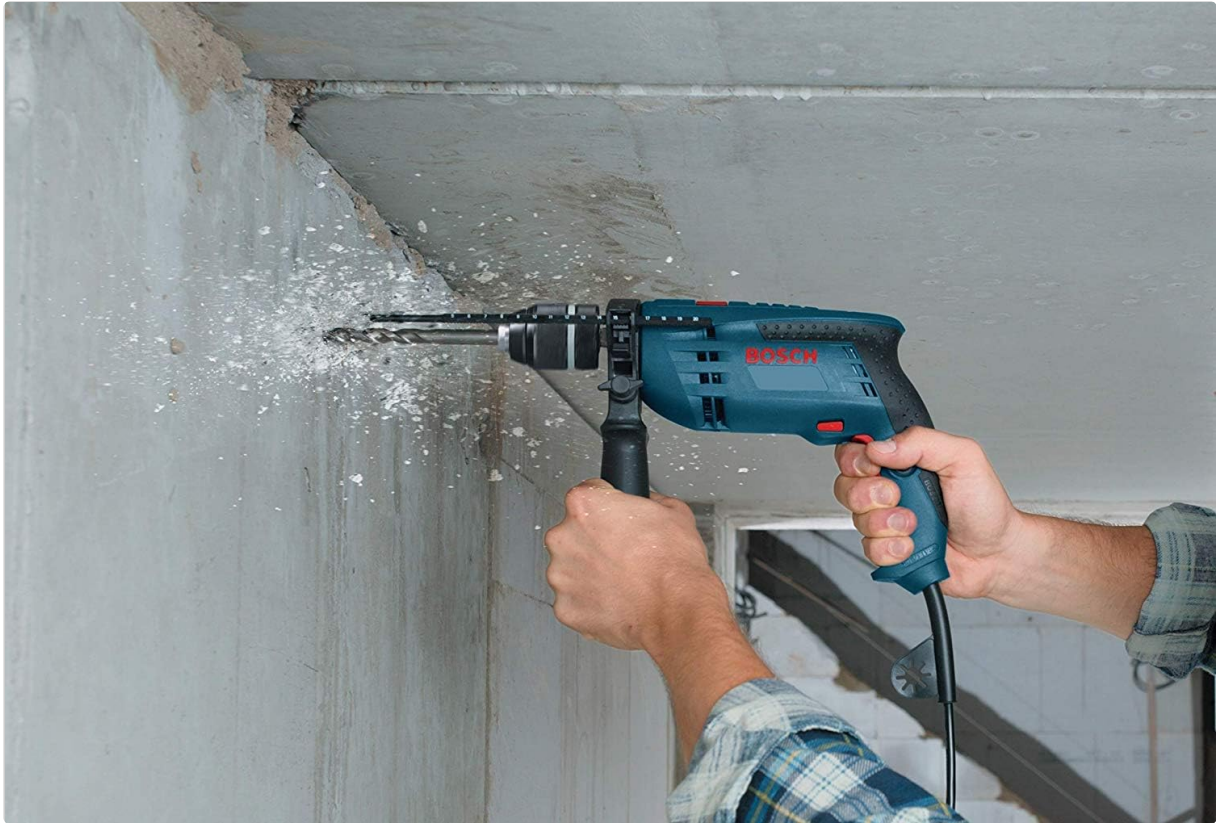
Figure 4: Depicts the hammer drill in action, demonstrating its capability to drill into concrete surfaces.
