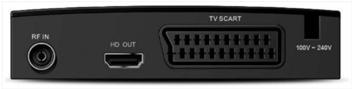
Image: Rear view of the AURA TDT Aries T2 receiver, showing RF IN, HD OUT (HDMI), TV SCART, and power input (100V-240V).
