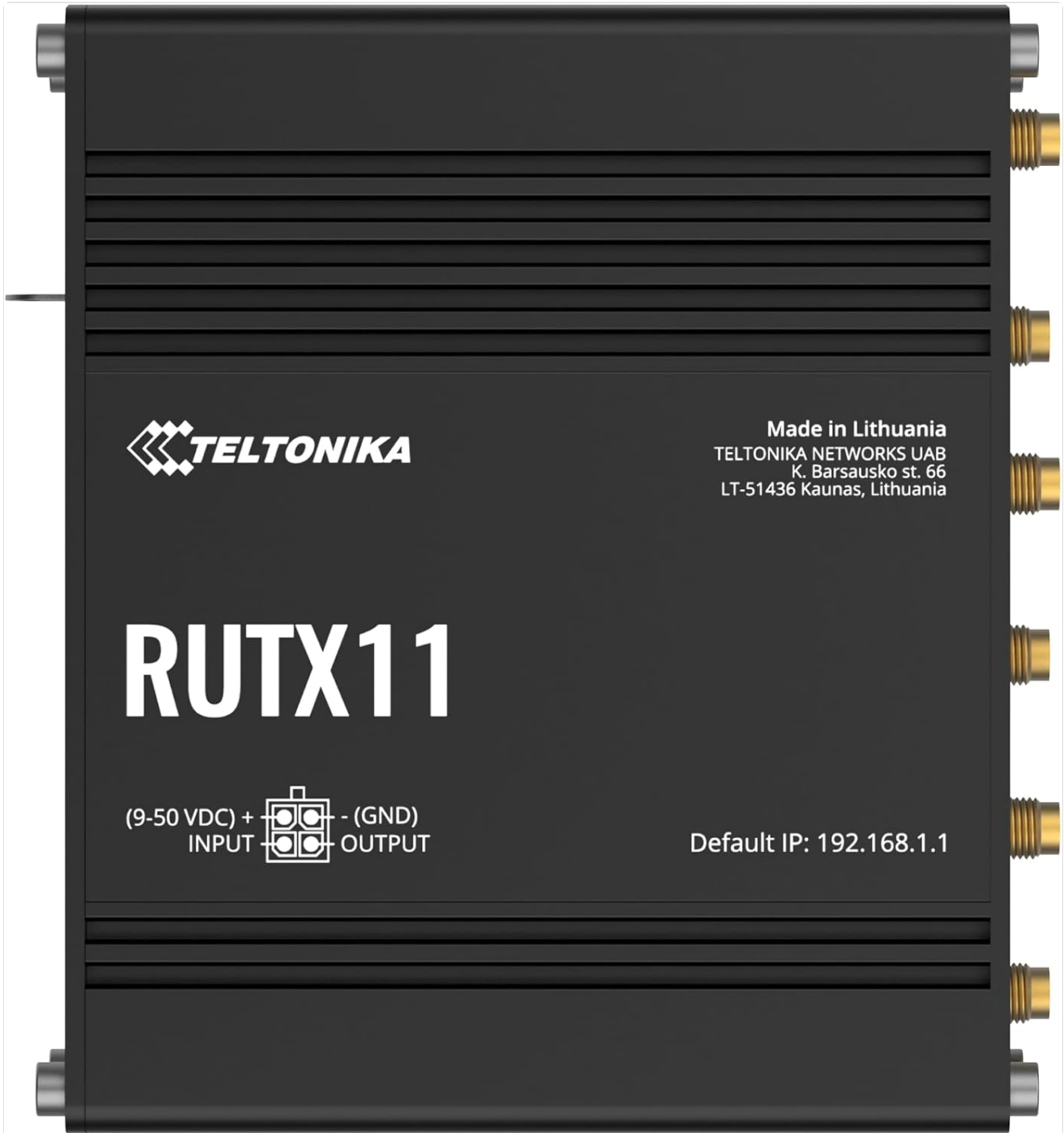
Figure 3.1: Front view of the Teltonika RUTX11 router, showing the brand logo, model name, power input, and default IP address.
