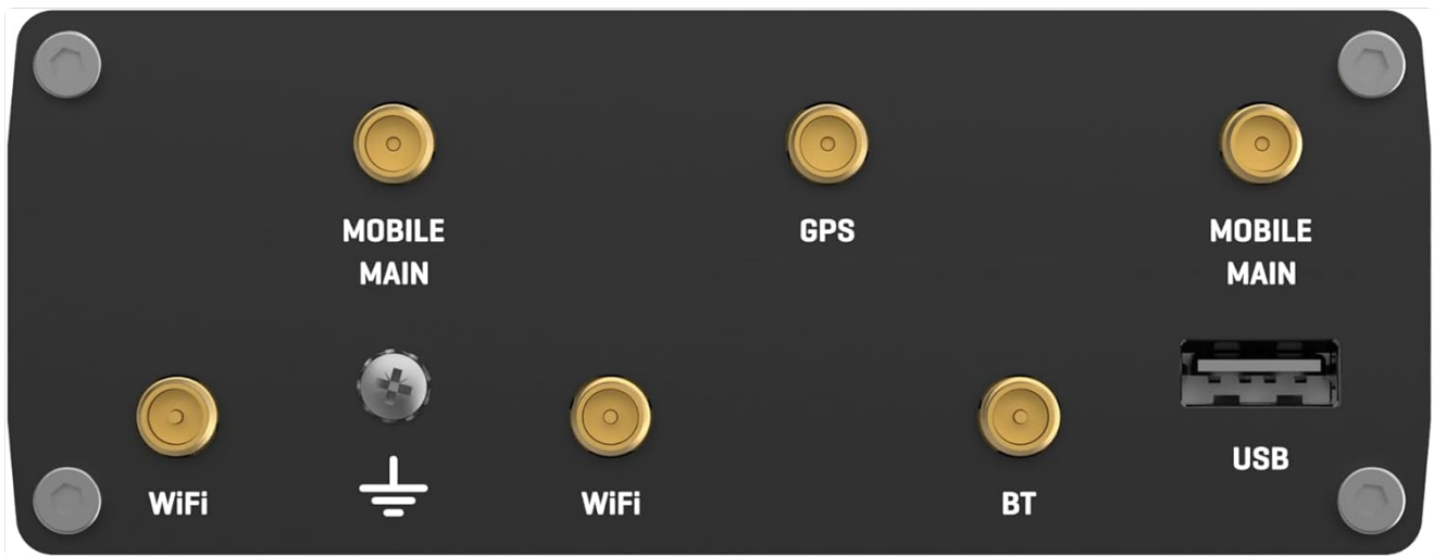
Figure 3.5: Detailed view of the RUTX11's rear panel. This shows the antenna connectors for Wi-Fi, Mobile Main (cellular), GPS, and Bluetooth, along with the USB port and grounding screw.
