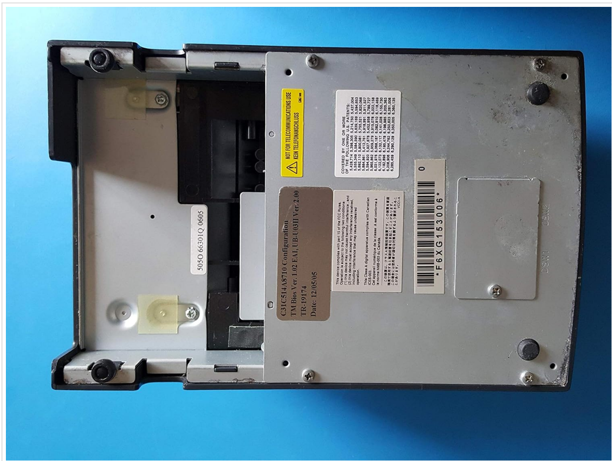
Figure 5: Bottom view of the Epson TM-U220B printer, revealing the panel covering the DIP switches. These switches control various printer settings and compatibility options.
