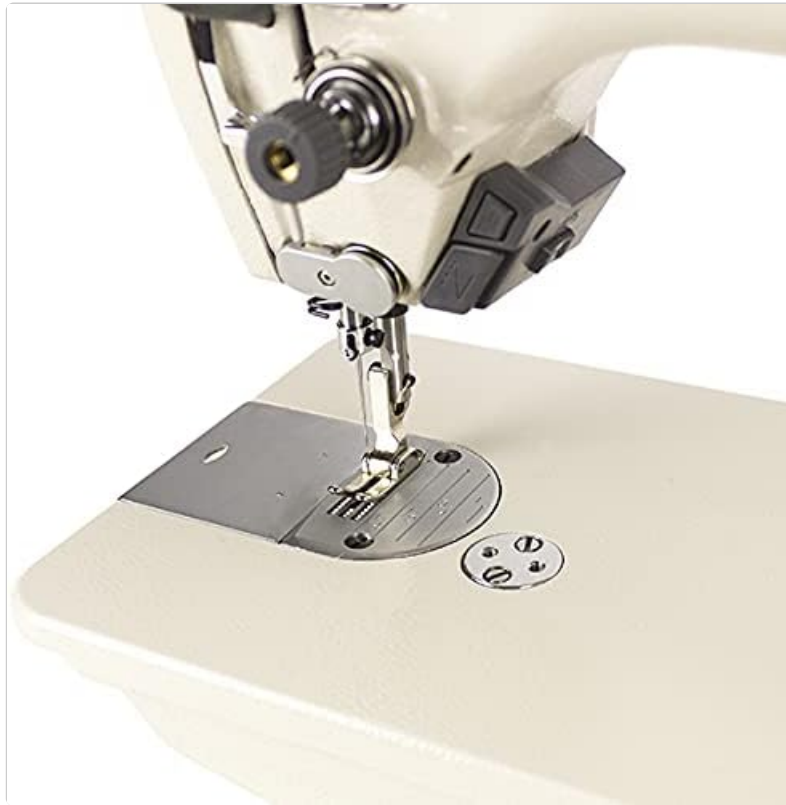
Figure 3: Detailed view of the needle bar, presser foot, and feed dogs. This area is crucial for fabric feeding and stitch formation.
