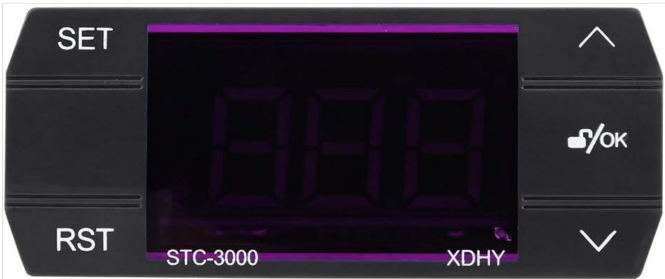
Figure 3: Front panel of the STC-3000 showing the digital display and touch buttons: SET, RST, Up arrow, Down arrow, and OK/°C/°F.
