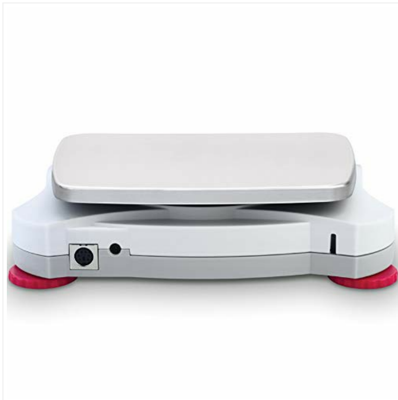
Figure 2: Rear view of the Ohaus Scout Portable Balance, illustrating the power input and optional communication ports.
