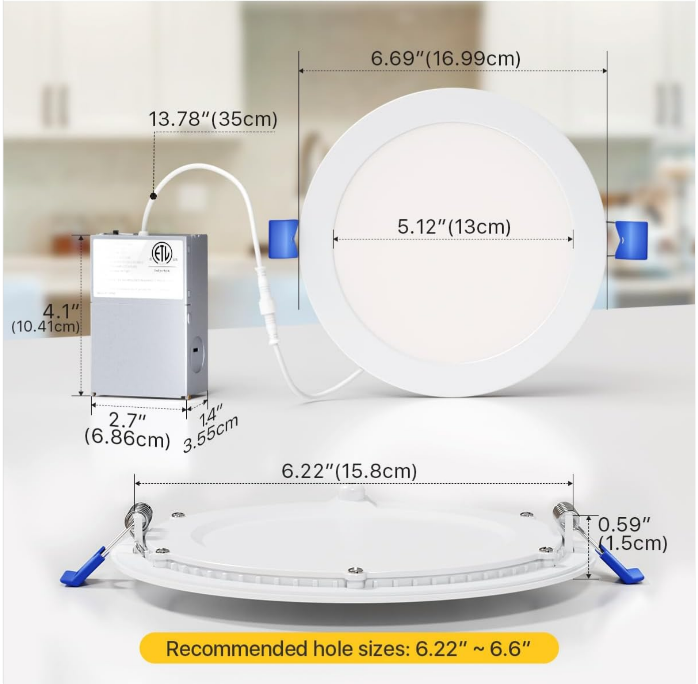
Image: Detailed product dimensions, including the light fixture and junction box, with recommended hole sizes for installation.
