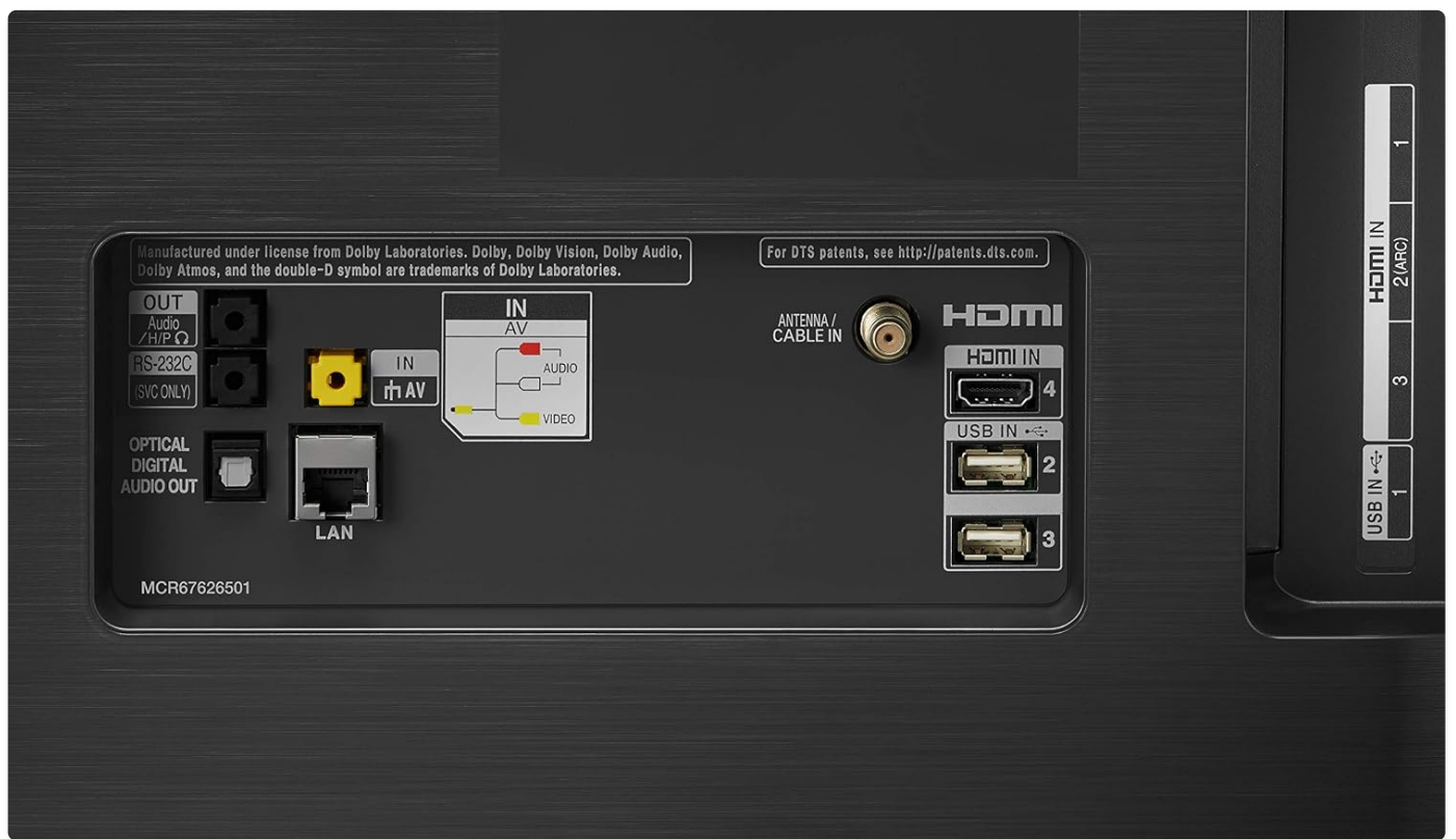
Figure 3: Rear input ports including HDMI, USB, LAN, and Optical Audio Out.
