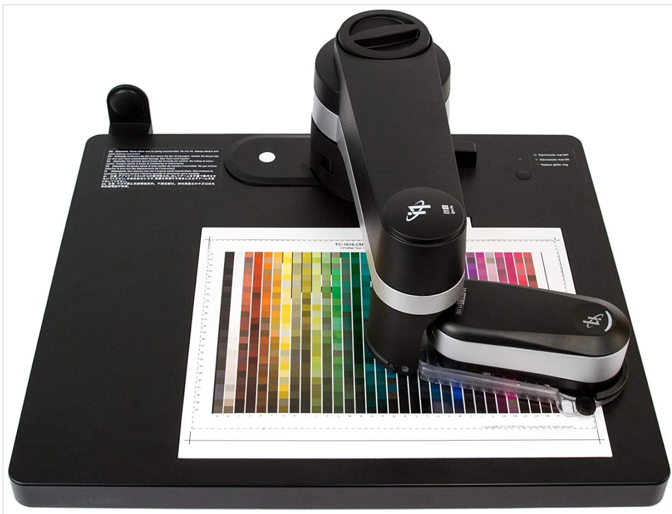
Figure 2: A detailed view of the X-Rite i1iO with the i1Pro 3 spectrophotometer securely attached to its robotic arm. The spectrophotometer is positioned directly over a color test chart, demonstrating its readiness to begin automated measurements. This image highlights the integration of the i1Pro 3 with the i1iO system.
