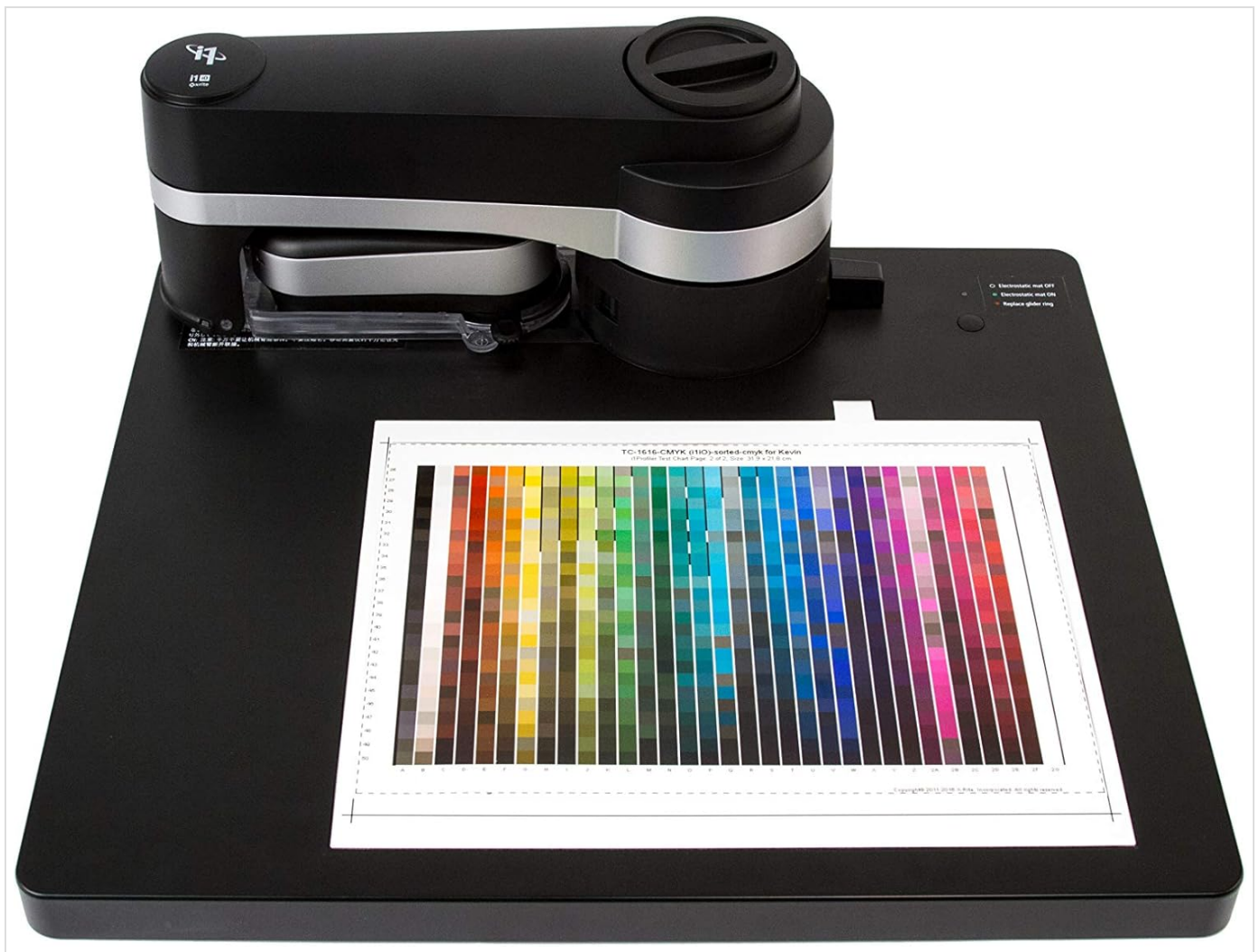
Figure 3: The X-Rite i1iO with a color test chart precisely positioned on its measurement surface. The chart is aligned within the designated area, indicating it is ready for the automated scanning process. This image illustrates the correct placement of a test chart before measurement.
