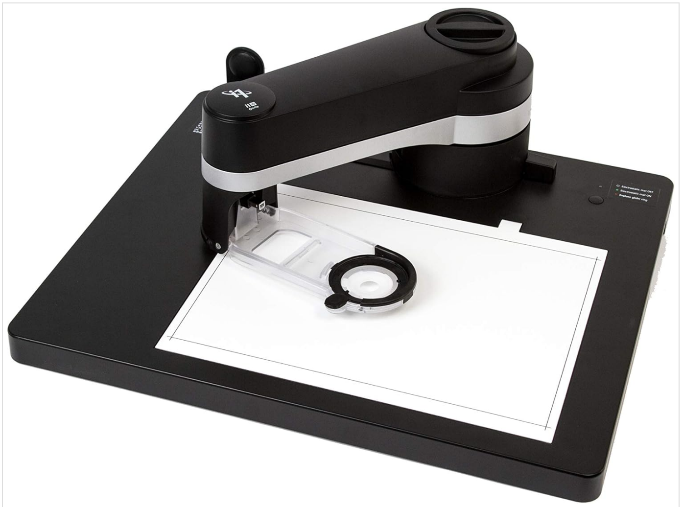
Figure 1: The X-Rite i1iO base unit with its robotic arm extended, ready for a measurement. A blank sheet of paper is positioned on the measurement bed, indicating the area where test charts will be placed. This image shows the general setup and footprint of the device.
