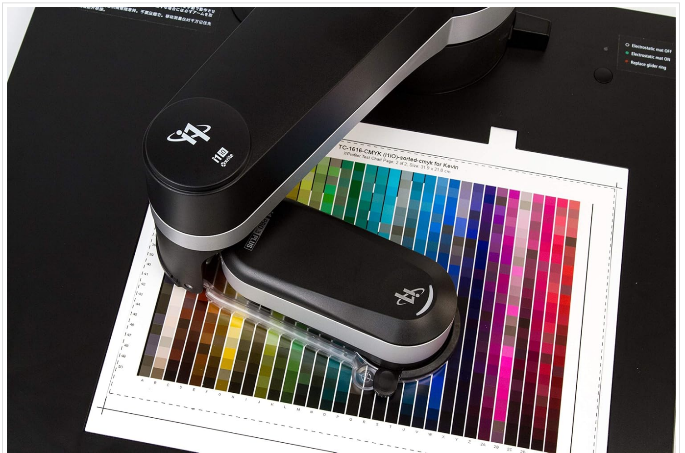
Figure 6: An overhead perspective of the X-Rite i1iO, showing the i1Pro 3 spectrophotometer resting on a color test chart. This view emphasizes the compact design and the precise positioning of the measurement head over the chart, indicating the completion of a scan or readiness for the next one.
