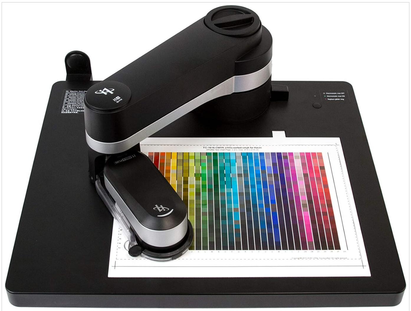
Figure 5: The X-Rite i1iO with its robotic arm in motion, performing a full scan of a color test chart. This image illustrates the automated movement of the spectrophotometer across the entire chart, highlighting the efficiency and hands-free operation of the system during the measurement process.
