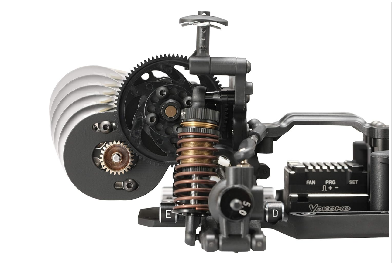
Image Description: A close-up side view of the assembled rear motor conversion unit, showing the motor, spur gear, pinion gear, and the new gearbox housing. The motor is positioned higher and further back than a standard YD-2 setup.
