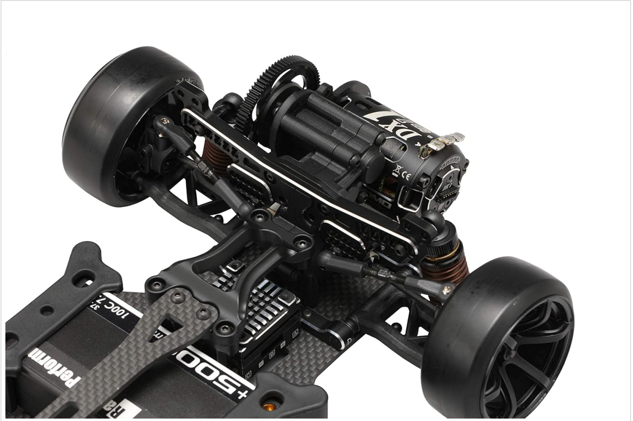
Image Description: A side view of a Yokomo YD-2 chassis with the rear motor conversion kit fully installed. The motor is prominently located at the very rear of the chassis, above the differential.
