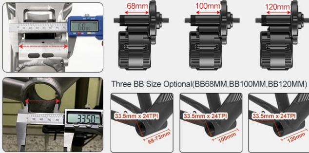
Figure 4.1: Guide for measuring your bike's bottom bracket to ensure compatibility with the BAFANG mid-drive motor. This image details the required length (68-73mm, 100mm, or 120mm) and internal diameter (33.5-36mm) for proper fitment.
