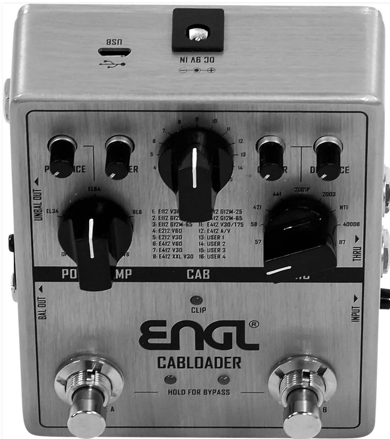
Figure 2: Rear view of the ENGL Cabloader pedal, highlighting the USB port for computer connection and the 9V DC power input. This view also shows the overall compact design of the unit.
