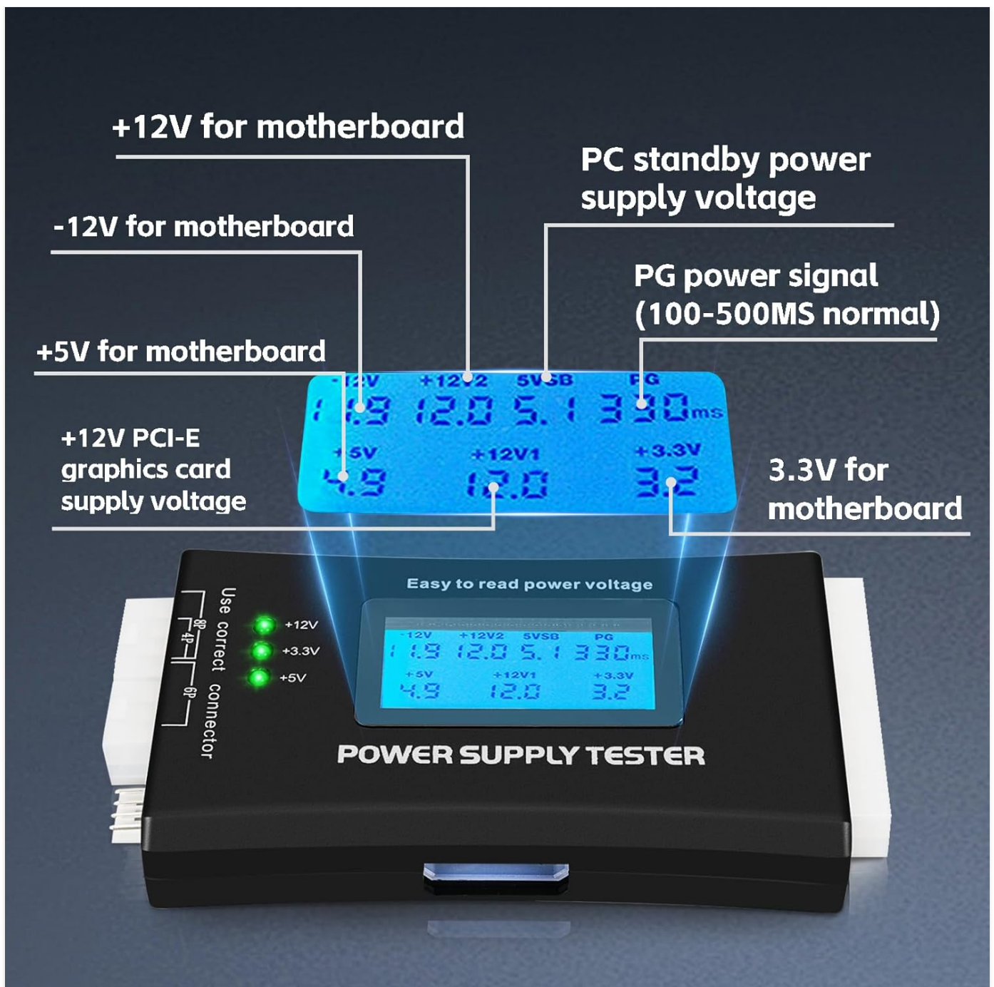
Image: A detailed breakdown of the voltage readings displayed on the LCD screen and their corresponding functions within a computer system.
