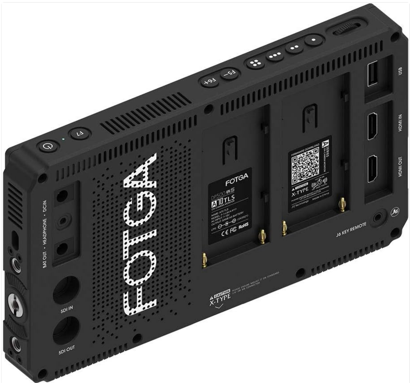
Figure 2.2.3: Rear view of the FOTGA A70T monitor, displaying the dual NP-F battery plates, USB port, HDMI IN/OUT, SDI IN/OUT, DC IN, and headphone jack. A QR code for firmware download is visible on the battery plate area.
