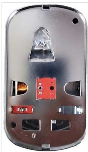
Figure 4.2: Rear view of the Trine #275 Sonnerie/Vibreur Bell. This image shows the back of the unit, revealing the internal components, wiring terminals (red blocks), and mounting brackets necessary for installation.
