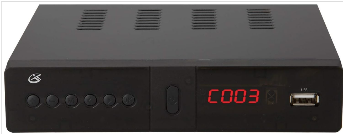
Figure 4.1: Front view of the GPX TVRT149B unit, showing the power button, channel navigation buttons, menu button, OK button, and a USB port on the right side.
