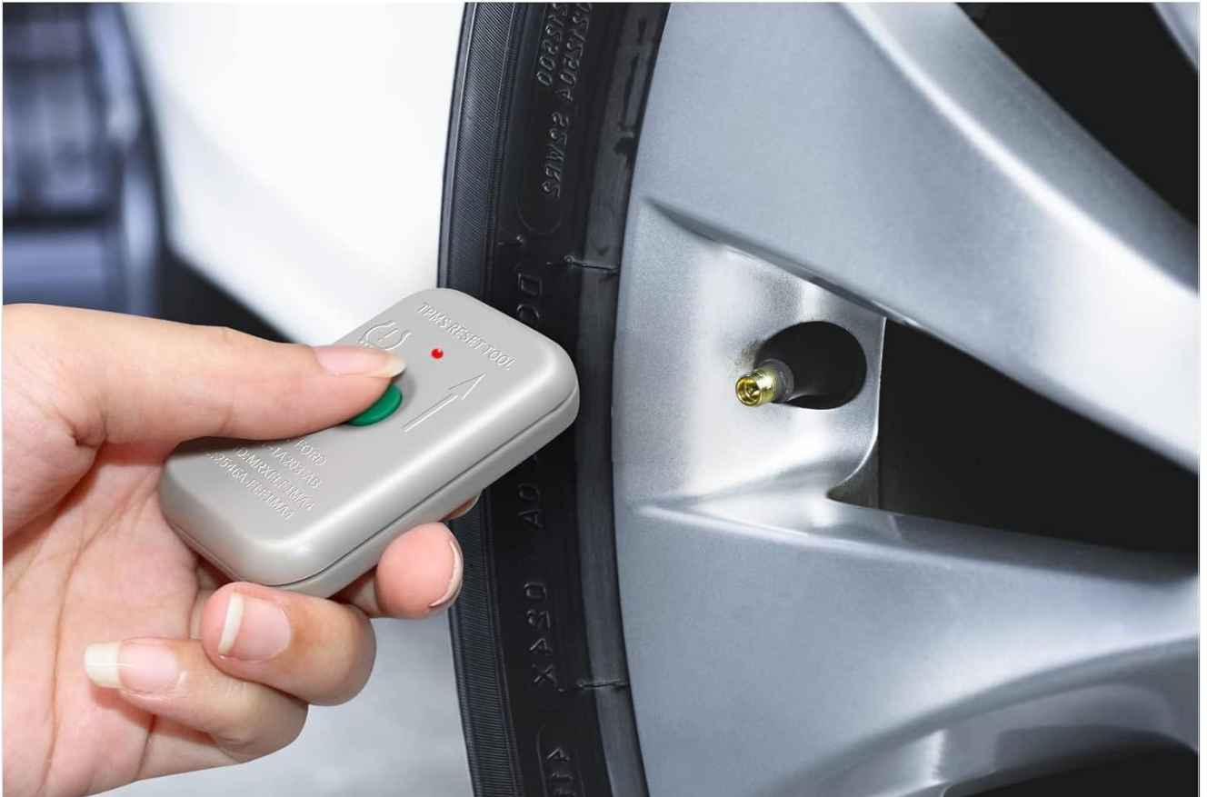
Image: Demonstrates the correct position to hold the TPMS relearn tool, near the tire's valve stem, for optimal signal transfer.
