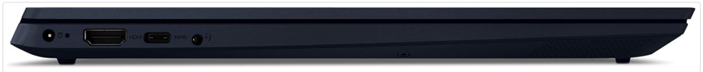
Figure 2.4: Left side of the laptop, featuring the power input, HDMI 1.4b port, one USB 3.1 Gen 1 port, and a 3.5 mm Headphone/Microphone Output jack.
