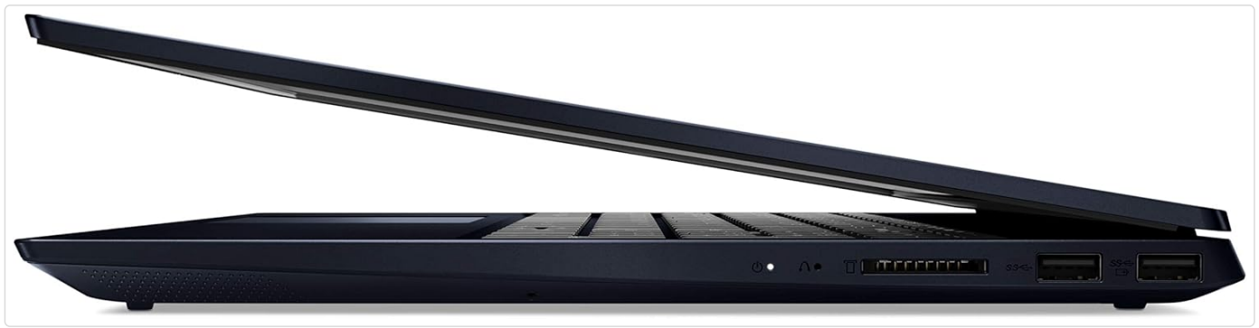
Figure 2.3: Right side of the laptop, featuring two USB Type-A (USB 3.1 Gen 1) ports and an SDXC/MMCplus Hybrid card reader.
