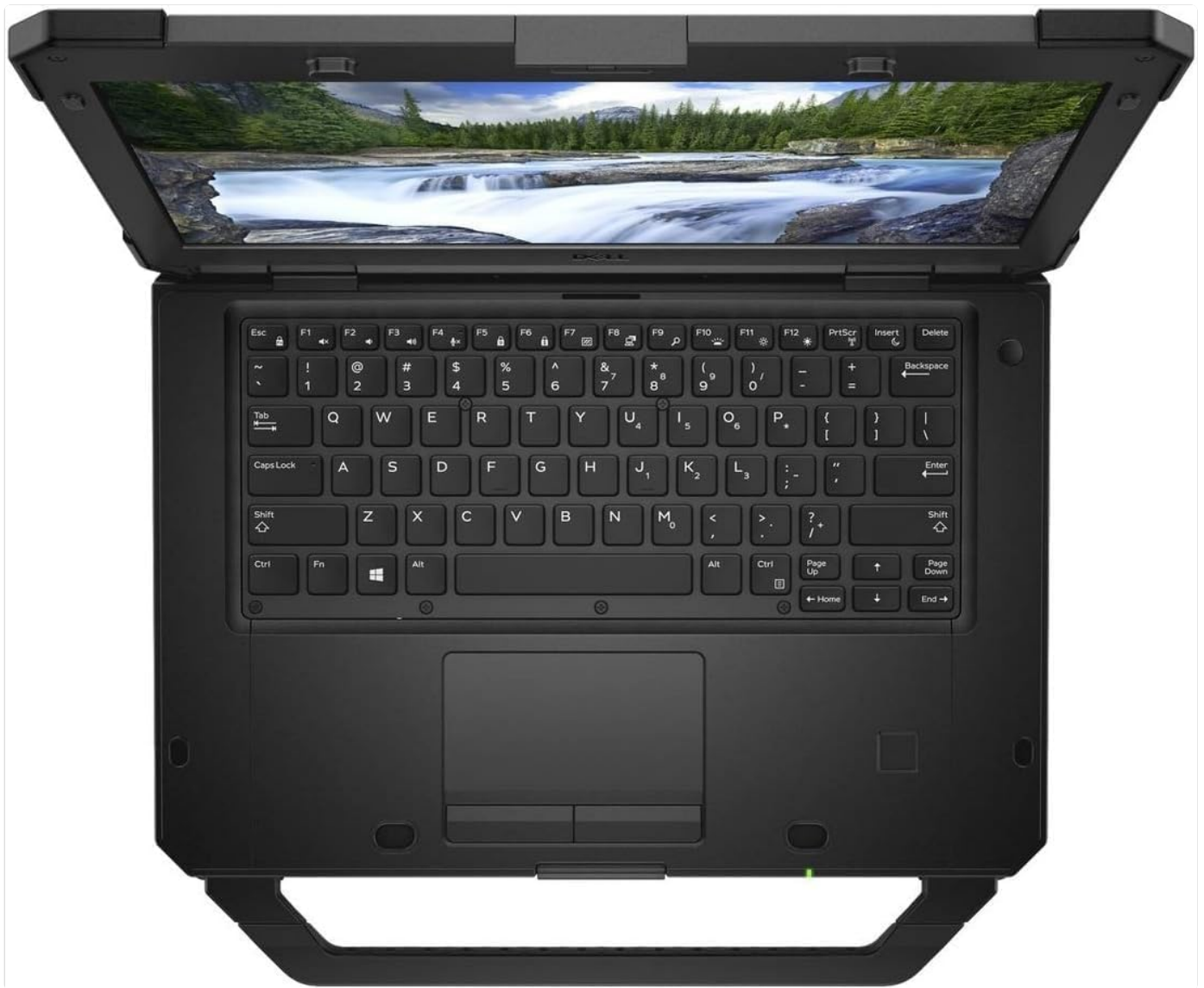
Figure 2: Top-down view of the Dell Latitude 5424 Rugged Laptop's keyboard and touchpad. This image highlights the layout of the keys, the integrated touchpad, and the ruggedized frame surrounding the input area.
