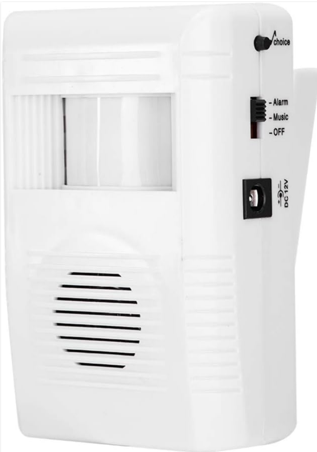
Figure 5: Detailed view of the mode switch, showing options for Alarm, Music, and OFF.
