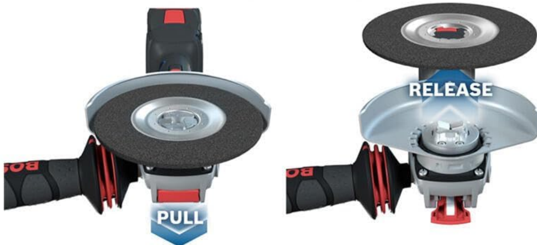
Figure 3.1: Quick accessory changes with X-LOCK system, illustrating snap-in mounting and single-lever release.
