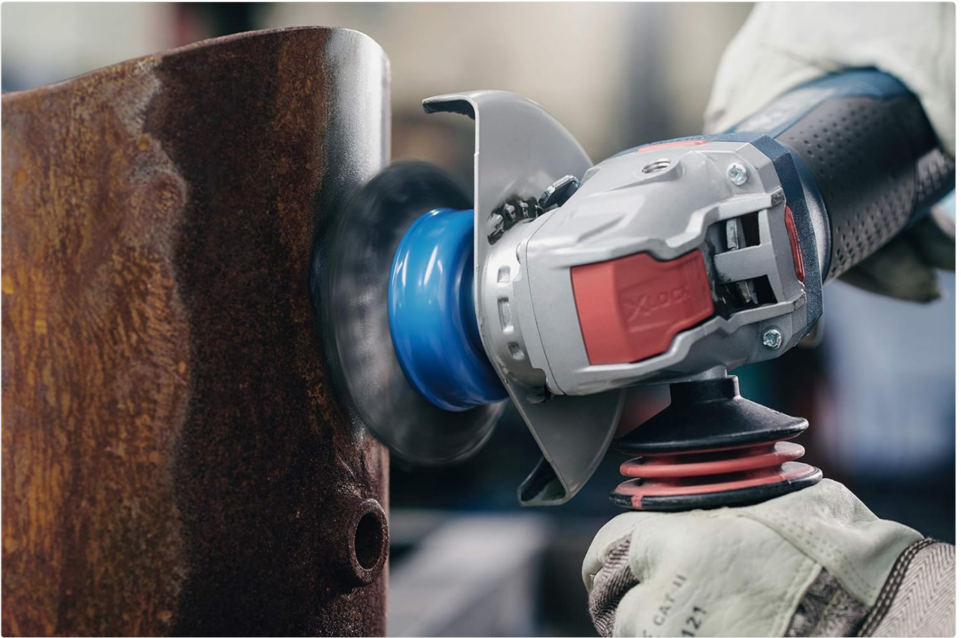
Figure 4.1: The BOSCH WBX319 wire cup brush in action, effectively removing rust from a metal surface.
